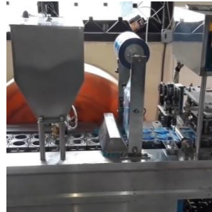
Gambar 5. Proses Cup Filling Machine
