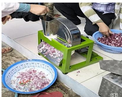
Gambar 2 Mesin Pengiris Bawang model vertical rotary
