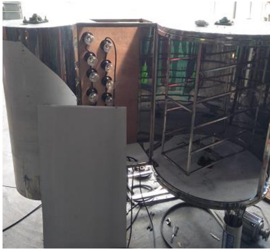
Gambar 4. Mesin Pengering "Food Dehydrator" Tipe Berputar
