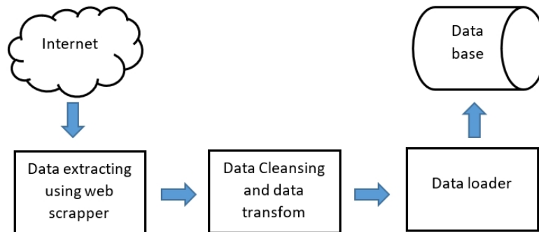
Figure 1. System Block Diagram
