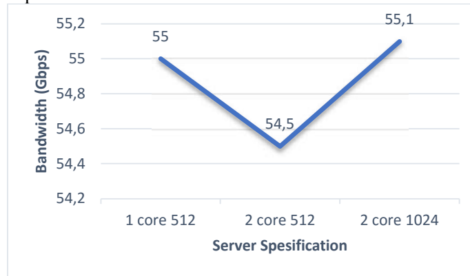
Figure 2. Performance of Linux Bridge measured using TCP protocol
