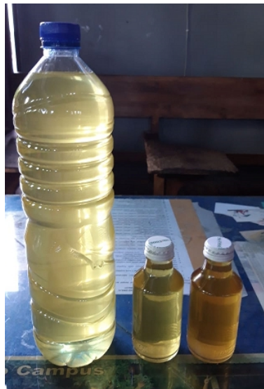
Figure 3. Polypropylene Fuel from Incinerator Pirolysis
