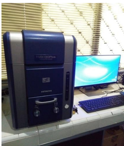
Figure 3. SEM (Scanning Electron Microscope) Hitachi TM3030Plus
